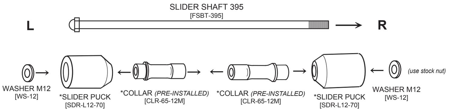
\* Slider Puck and Collar are sold with together as a single part, with the Collar pre-installed inside the Slider Puck.
